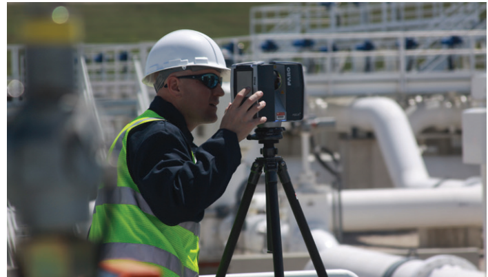
Figure 1: Laser scanning in operation. 3D laser scanning provides a tool that enables engineers and designers to think, design and evaluate in a three dimensional world with even greater ease.
